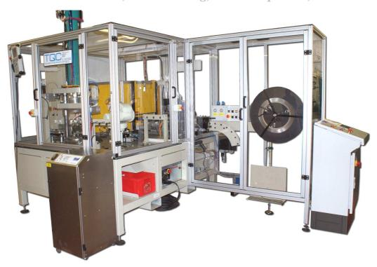
TQC have designed and manufactured a fully automatic manufacturing cell for the production of laser welded metal rings.
